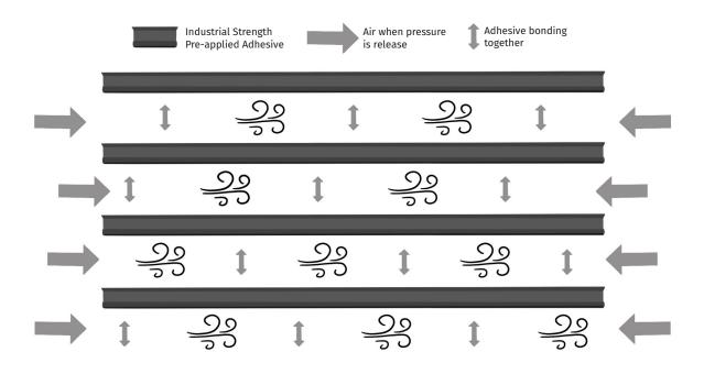
Factory-applied adhesive is applied in groups of parallel string, with airspaces between each string of adhesive. When pressure is applied using the installation tool, the air between the glue strings is forced out, and a soft "suction" is created when the pressure is relieved.
